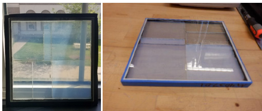
Figure 15. Prototype 26.7 \times 26.7 \times 1.8 cm aerogel IGU fabricated using 0.5 cm thick silica aerogel monoliths packaged between two 6.35 mm thick glass sheets.
