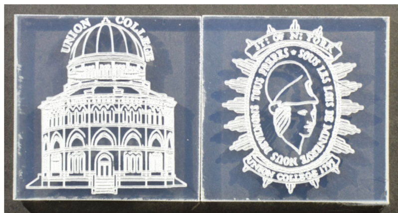
Figure 11. Photographs of 5 \times 5 \times 0.5 cm laser-cut and etched silica aerogel monoliths. These aerogel samples were photographed on top of black flocked paper.
