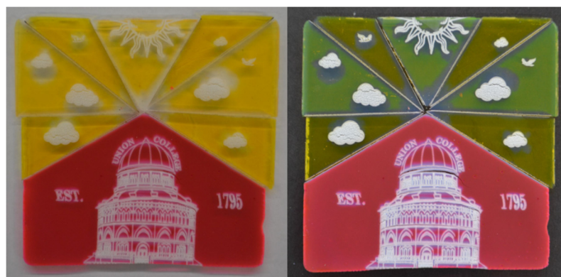
Figure 13. Stained-glass design prototype consisting of a combination of aerogel pieces laser-cut and -etched from different dye-containing 0.5 cm thick monoliths for subsequent incorporation into a window prototype. The length dimension at the bottom of the largest piece is 12.5 cm. Photographs were taken of the aerogel assembly on white ( left ) and black flocked ( right ) paper.
