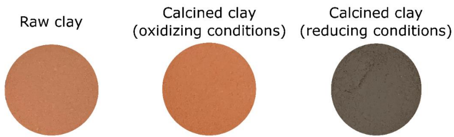
Figure 10: Colour of raw and calcined iron-oxide containing (3.8 wt.%) kaolinitic clay under oxidising conditions and reducing conditions. Adapted from ref [22, 129].
