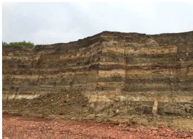
Figure 1: Photograph of a stockpile with layers of different types of clays, which can then be extracted by digging vertical slices from the stockpile to homogenise the clays.
