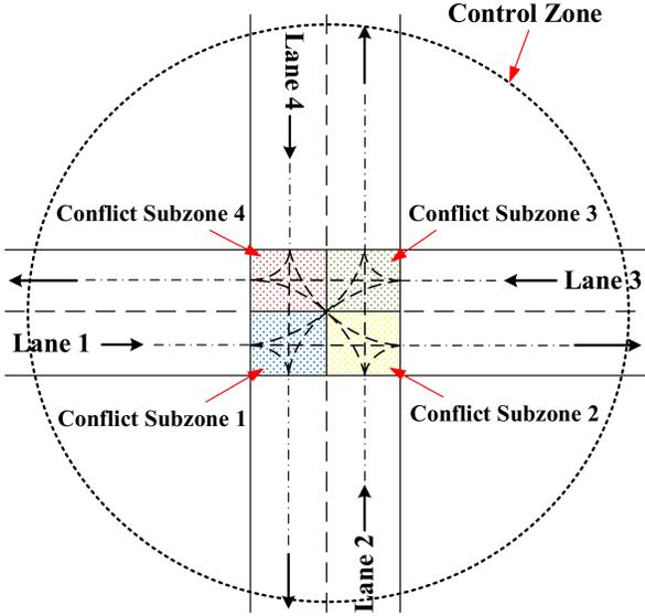
Fig. 1. A typical intersection.
