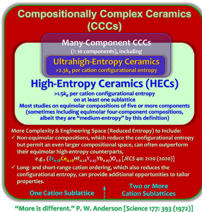
Fig. 1 Schematic illustrations of high-entropy ceramics (HECs) and compositionally complex ceramics (CCCs), along with the proposed many-component CCCs and ultrahigh-entropy ceramics. Following a convention commonly used in high-entropy alloys [50], we can define HECs to refer to ceramics possessing > 1.5k_B per cation ideal configurational entropy on at least one sublattice [1], where k_B is the Boltzmann constant. Most prior studies of HECs focused on equimolar compositions of five or more components, but some studies also included equimolar four-component compositions, albeit they are “medium-entropy” by this definition [1]. We also proposed to broaden HECs to CCCs to include medium-entropy and/or non-equimolar compositions and consider long- and short-range cation ordering, which reduce the configurational entropy but provide additional opportunities to tailor properties [1]. Many-component CCCs ( \geq 10 components) offer further compositional complexity (and tunability). Moreover, we can define ultrahigh-entropy ceramics (a subclass of HECs and a subclass of many-component CCCs) as those HECs with > 2.3k_B per cation ideal configurational entropy on at least one sublattice; noting that \ln 10 \approx 2.3 , so that equimolar many-component CCCs with \geq 10 disordered (randomly dissolved) components should be ultrahigh-entropy. We note that these definition thresholds adopted here (5 vs. 10 components and 1.5k_B vs. 2.3k_B per cation) are somewhat arbitrary and subjective. Like HECs vs. CCCs, non-equimolar compositions and cation ordering can reduce the configurational entropy of many-component CCCs so that they (may or) may not be ultrahigh-entropy (or even high-entropy) ceramics. Two or multiple cation sublattices, anion mixing, mixed ionic–covalent–metallic bonding, and defects (e.g., oxygen vacancies and aliovalent doping) can further increase the complexity of CCCs. It is important to note that maximizing the entropy may not always be beneficial or necessary; the complexities in (many-component) CCCs offer more opportunities to tailor properties, where different or new phenomena can be emergent in complex systems, because “more is different” [52].
