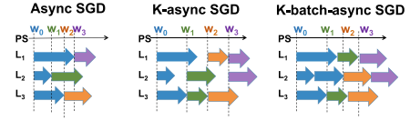
Fig. 5. For K = 2 and P = 3 , we illustrate the K -async and K -batch-async algorithms in comparison with fully asynchronous SGD.
