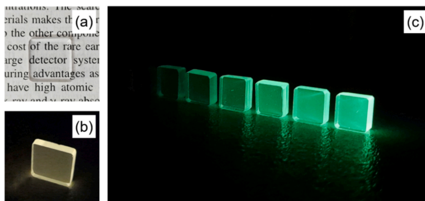
Fig. 2. Photographs of the undoped glass under (a) ambient light, and (b) UV excitation (326 nm). (c) Photographs of the \text{Tb}^{3+} doped glasses under UV lamp excitation (376 nm), in ascending order of Tb-concentration (0.5, 1.0, 3.0, 5.0, 7.0 and 10.0 mol%) from left to right.
