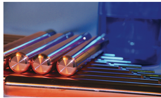
(b) Copper cylinders from electroformation
