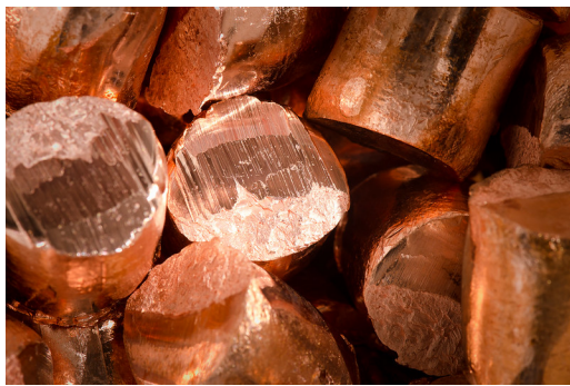
(a) Copper nuggets prior to electroformation
