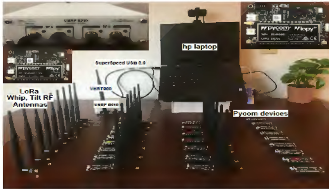
Fig. 1: IoT Testbed: 25 Pycom devices and USRP B210.
