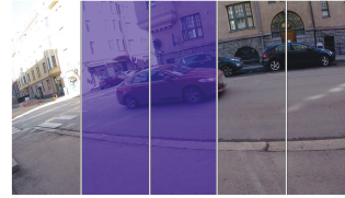
Fig. 2. Left: Regions activated using the full bounding box, Right: regions activated using the bounding box center. Each region conveys 24^\circ . Note: black vehicle is parked so it is not annotated.
