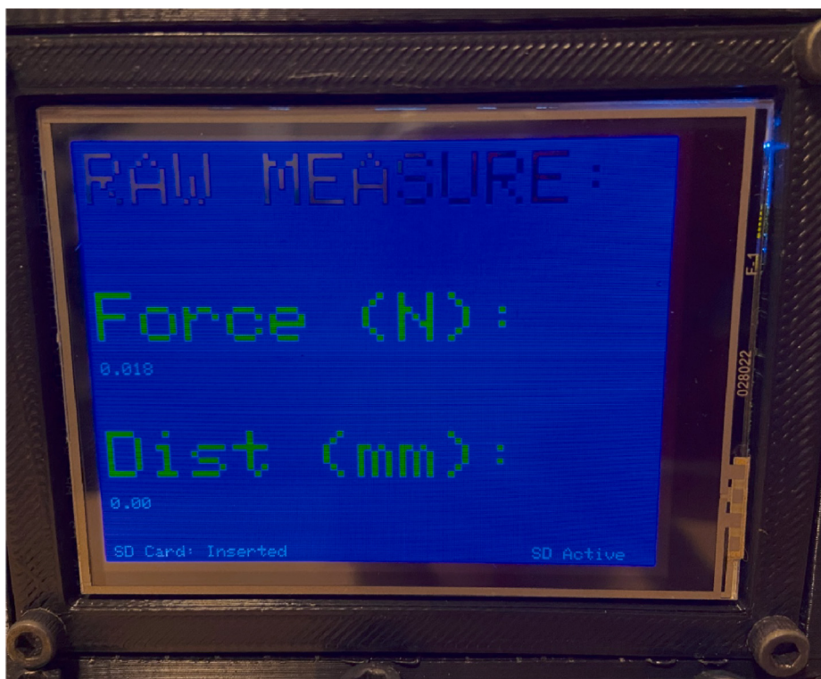
Fig. 71. The Raw Measure Screen (SI units).
