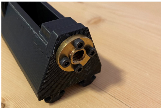
Fig. 31. The Lead Screw Nut has been secured to the Load Cell Carriage.
