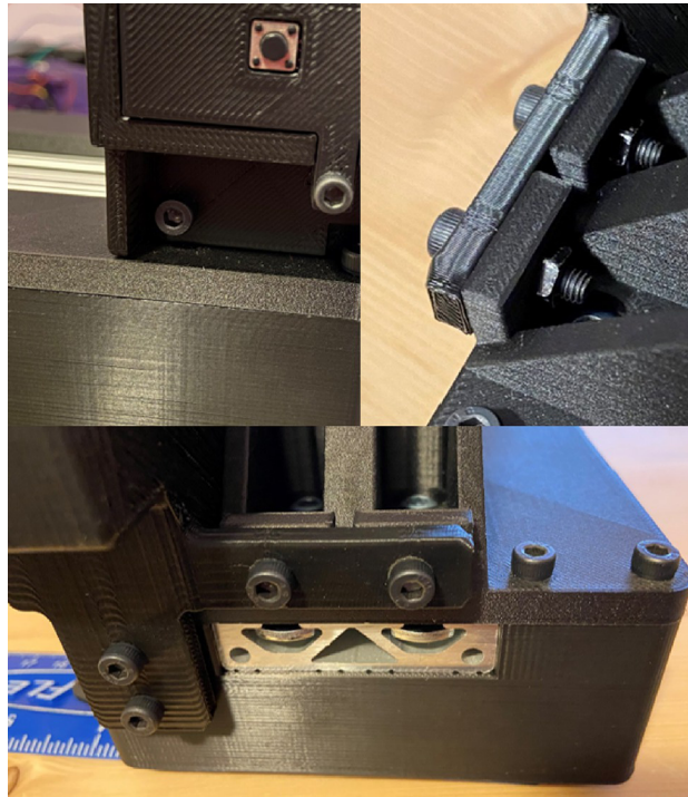
Fig. 30. TOP LEFT shows a single 4\text{ M} \times 0.7\text{ 16 mm} bolt connecting the D-Pad Housing to the Battery Cover. TOP RIGHT shows two 4\text{ M} \times 0.7\text{ 16 mm} bolts connecting the D-Pad Housing to the Battery Cover. The bolts are secured on the backside by two 4\text{ M} \times 0.7 bolts. BOTTOM shows two 4\text{ M} \times 0.7\text{ 10 mm} bolts on the bottom left connecting the D-Pad Housing to the Battery Housing.
