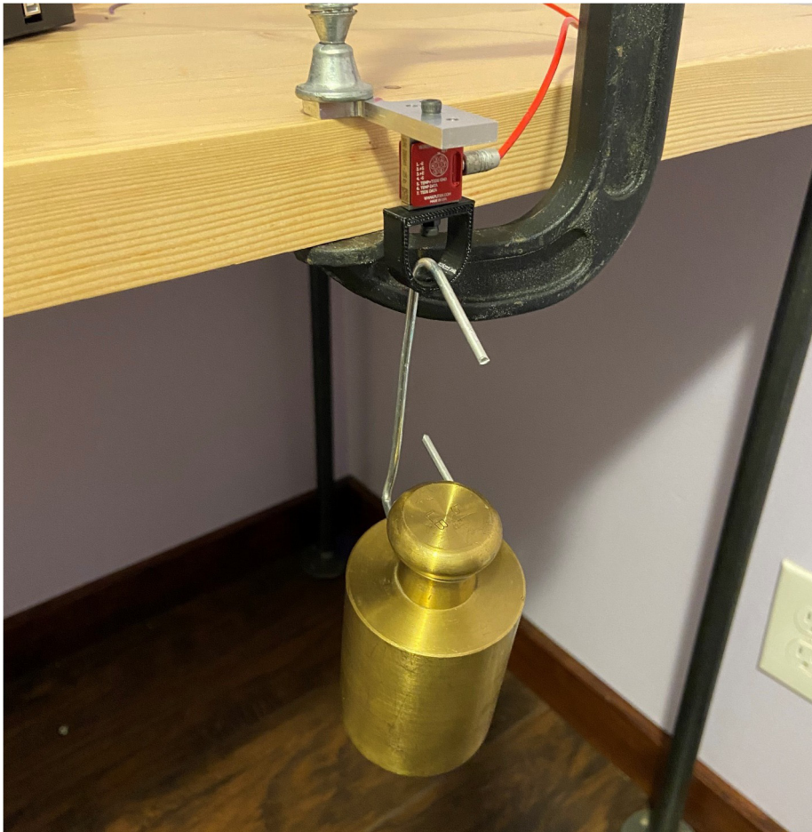
Fig. 81. A mass hanging from the Calibration Piece.
