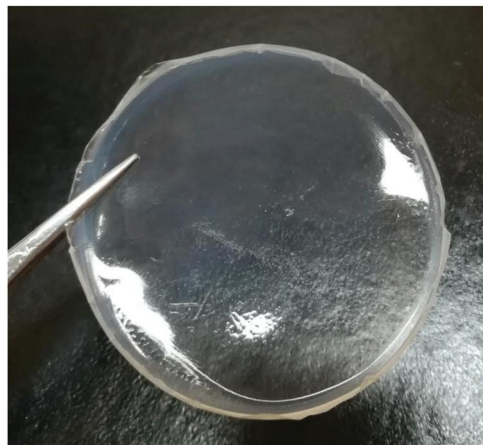
Fig. 2 Image of the BMPyr-TFSI free standing film using 10 wt% PBDT and 90 wt% IL. Each film was controllably produced with a thickness of 100–200 \mu\text{m} , tailored to suit the needs of the characterization methods employed.
