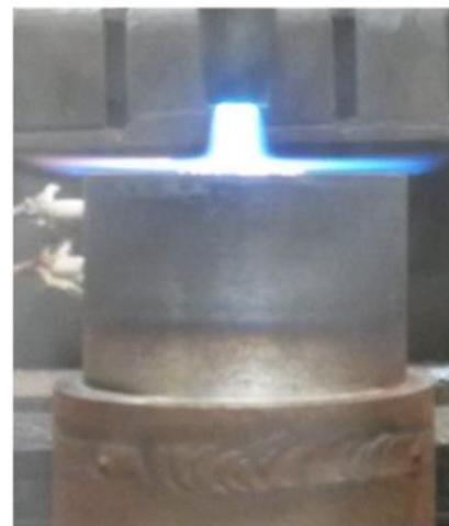
FIGURE 1: Oxyfuel cutting preheating process experiment [1].
