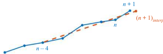
Figure 5. Predictive tracking schematic. The solid line signifies the real trajectory. The dotted line (linear fit of the positions from frame n - 4 to n ) indicates the position extrapolation.
