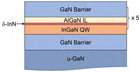
Fig. 1. Novel active region design consisted of an InGaN QW, \delta -InN and AlGaIn interlayer between GaN barriers.
