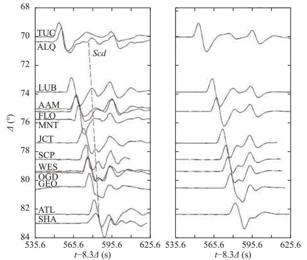
**Figure 4.** Profile of digitized WWSSN SH component recordings for the 29 January 1971 event (left panel) showing the systematic move-out with increasing epicentral distance,  $\Delta$ , for the extra arrival between S and ScS seen in Figure 3, which we labeled Scd. Generalized ray theory synthetics for a model with a 2.75% shear velocity discontinuity at the top of the D'' layer are shown on the right, matching the primary features of the observed signals. From Lay and Helmberger (1983d).
