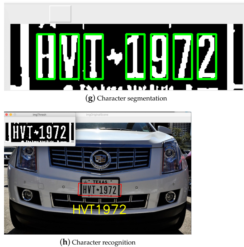
Figure 2. Phases of the plate detection, character segmentation, and recognition modules.
