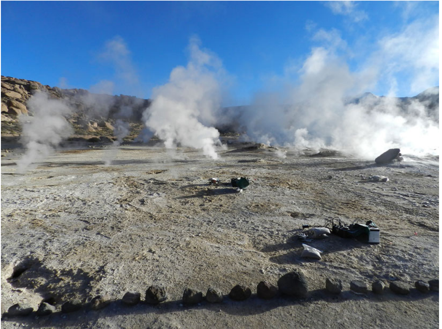
An array of instruments (foreground) measures seismic tremor around geysers at El Tatio in Chile. Credit: Shaul Hurwitz, U.S. Geological Survey
