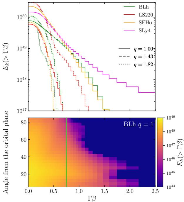
**Figure 3.** Cumulative kinetic energy distribution for a selected set of models (*top panel*) and its angular distribution for a BLh  $q = 1.00$  model (*bottom panel*). The vertical light green line marks the  $v_{ej} = 0.6$ . The top panel shows that equal mass models have a more extended high energy tail, while the bottom panel shows that the angular distribution of the ejecta is not uniform.
