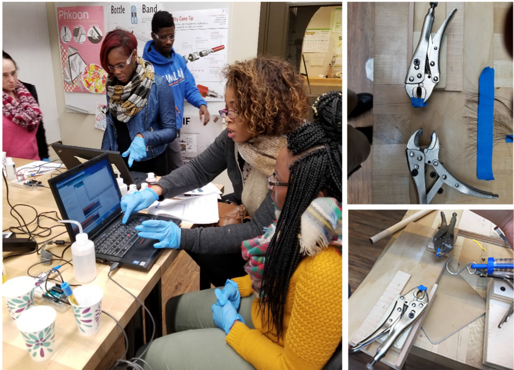
Fig. 9. Dry run of pH sensors with hair stylists (left); DIY tensile strength of hair tester (right).
