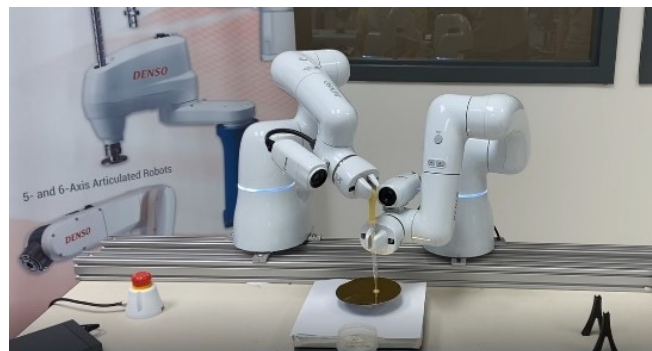
Fig. 1. Next-generation intelligent robots are highly portable, can work collaboratively with human operators and have the ability to self-learn.
