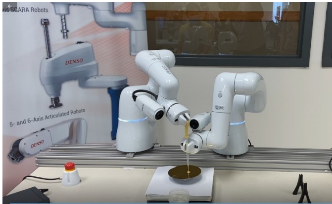
Fig. 5. Intelligent robots are compact in size, light weight, and equipped with machine vision systems and can move payloads with high precision and accuracy.
