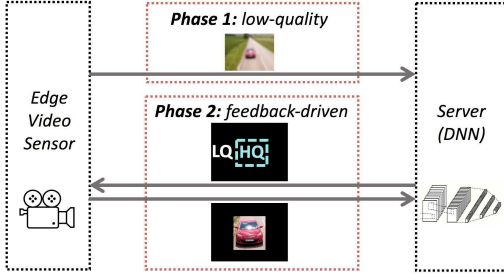
Figure 1: A typical server-driven video analytics workflow. LQ refers to low encoding quality and HQ refers to high encoding quality.
