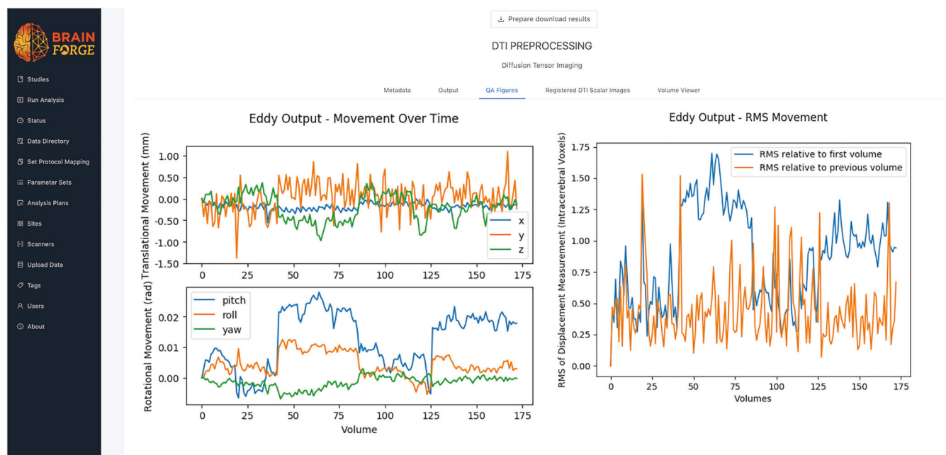
FIGURE 1 QA measures produced by DTI pipeline related to movement as provided by FSL eddy program
