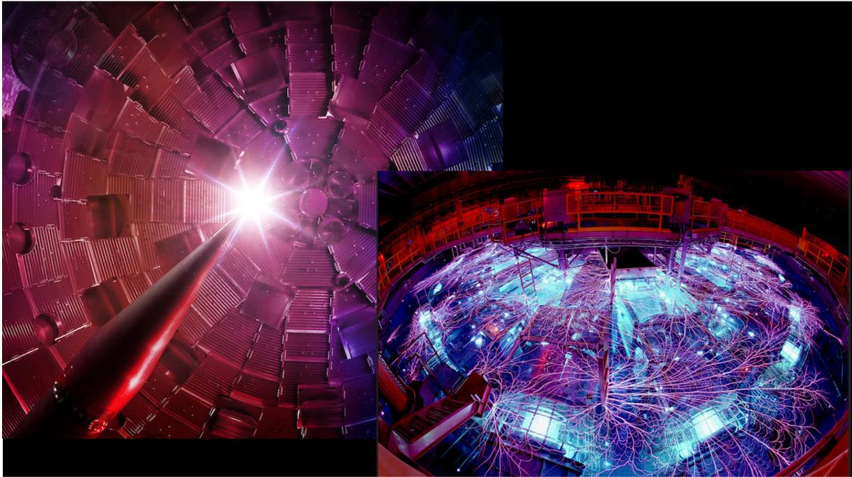
**Fig. 1.** Measurements at the National Ignition Facility (NIF, *left*) and the Z pulsed-power facility (*right*) provided the means of calibrating high-pressure experiments to terapascal pressures. The spherical target chamber at NIF is 3 stories high (10 m), and the diameter of the Z machine is nearly 4 times larger (37 m).
