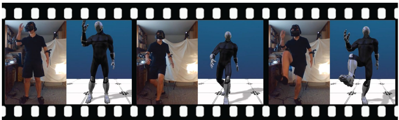
Fig. 5 A schematic showing side-by-side comparisons of the user and the avatar in different postures in real-time. Note that the avatar tracked the user's postures reasonably well without any noticeable differences
