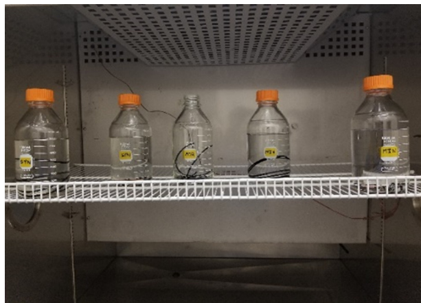
Fig. 2 The environmental chamber containing the synthetic and mineral oil jars with components
