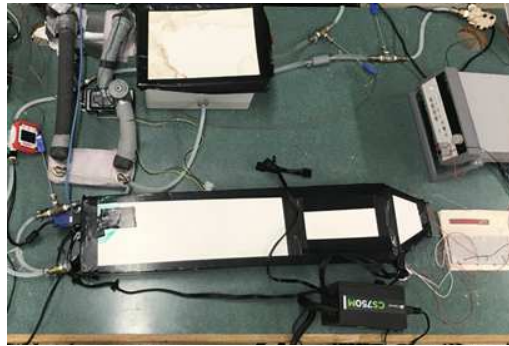
FIG. 3: Experimental setup showing the server cooling loop, pump control circuitry, and instrumentation for data acquisition
