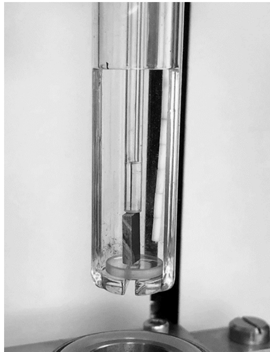
FIG. 10: Megtron6 PCB sample mounted on the TMA for testing
