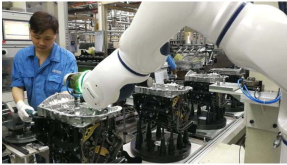
Fig. 2. Collaborative robot working with a human to assemble an engine. [31].
