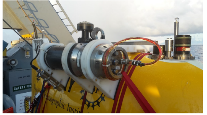
Fig. 4. The OWTTIUSBL test article mounted on the NDSF AUV Sentry for field trials in 2018. An iXBlue Phins fiber-optic north-seeking gyrocompass is rigidly mounted to one endcap of the housing. Several candidate AHRSs and the array were mounted to the same endcap to enable precise comparison of the AHRS data to ground truth provided by the Phins and to transform array angles into local-level coordinates.
