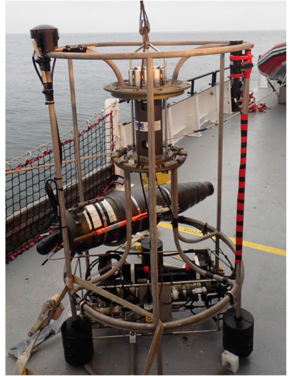
Fig. 5. Data from glider “lowerings” were collected with the Seaglider hull strapped to the inside of the CTD rosette frame, seen here on the far side of the rosette frame, with the iUSBL mounted on the top rail (upper left).
