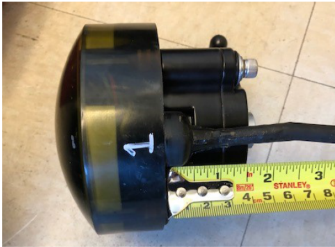
Fig. 3. The OWTTIUSBL head consists of the array with integral preamplifier with a small housing containing a MEMS AHRS rigidly bolted to its underside. The acoustic processing electronics were located inside the Seaglider's main pressure housing.
