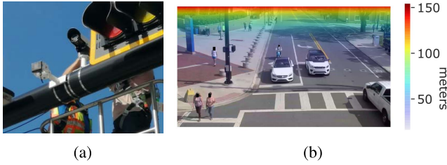
Fig. 4. a) Multi-sensor mounting configuration. b) Inspection of the estimated camera calibration matrix \mathbf{P} by visualizing world space distances from the camera for each pixel.
