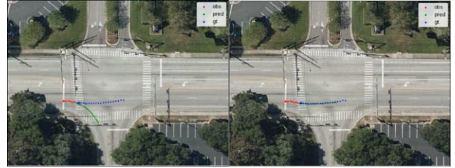
Fig. 9. Two predictions at inference time. The red, blue and green points represent observed, ground-truth future, and predicted points of a trajectory respectively.
