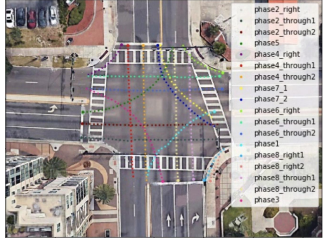
Fig. 6. The resulting prototypes. Note that the slight deviation of some prototypes is caused by imperfect Google Map alignment.
