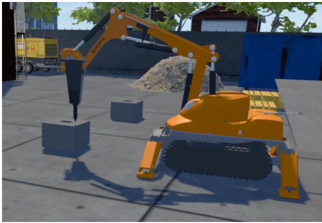
Fig. 1b. Simulated Brokk demolition robot.
