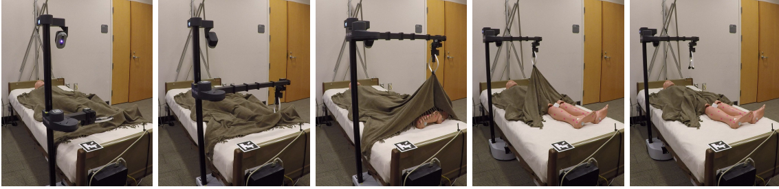
Fig. 4. Image sequence from executing a simulation-trained PPO policy to uncover both lower legs in the real world. The robot previously observed the pose of the manikin, as shown in Fig. 3. Sequence from left to right: 1) locate fiducial tags on opposite ends of the bed, 2) move end effector to the grasp location and grasp the blanket, 3) raise the blanket 40cm up from the top of the bed, 4) move linearly to the release location, 5) release the blanket.
