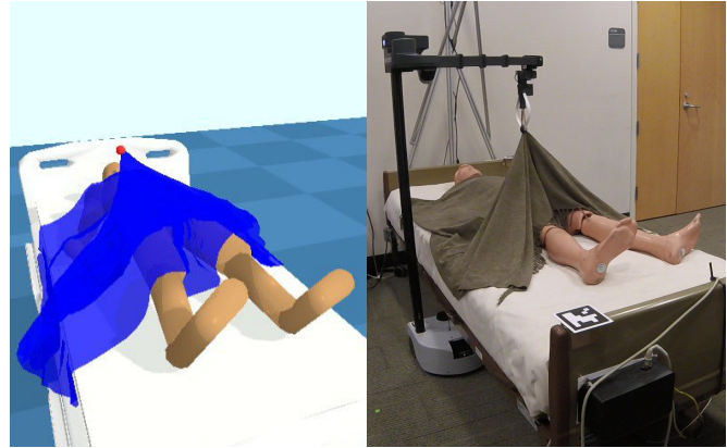
Fig. 1. A bedding manipulation policy trained in simulation that we have transferred to the real world for manipulating blankets over a person. (Left) The physics simulation environment used to train models for manipulating deformable blankets over a person. (Right) A real mobile manipulator (Stretch RE1) executing the simulation-trained policy to grasp a blanket and uncover the legs of a medical manikin.
