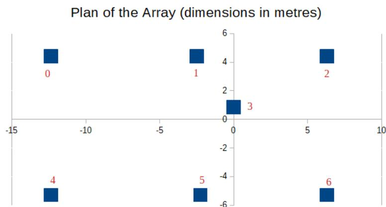
**Figure 1.** Plan view of the array. The scintillators are one metre squared, as indicated to scale on the diagram. For later reference, these detectors are labelled (red) as follows: top row, left to right, 0, 1, 2; middle detector, 3; bottom row, left to right, 4, 5, 6.
