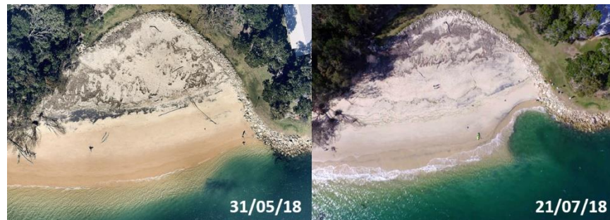
Figure 5: Typical Pre-Failure (Left) and Failed (Right) Beach, Source: NearMap & Drone Imagery
