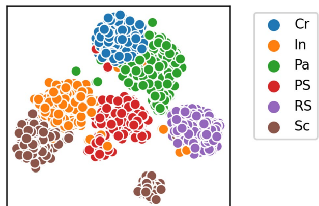
Fig. 10 t-SNE projection of feature data extracted from block5_pool layer from VGG16 with 110 unwhitened PCA components
