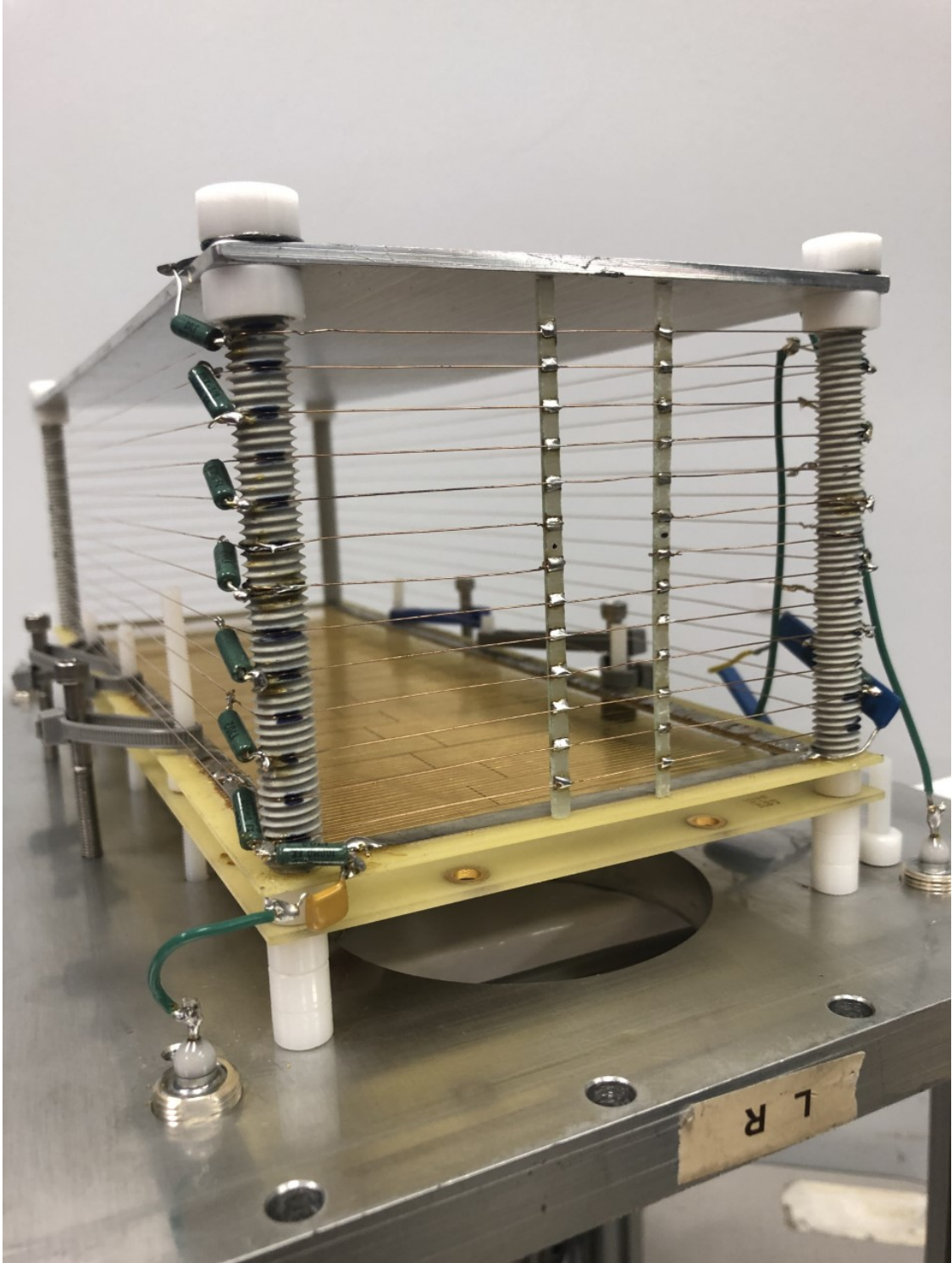
Figure 1: A picture of the active elements of the Encore detector. It consists of a cathode at the top and the segmented anode at the bottom (when mounted the detector sits upside-down to the picture's orientation). A Frisch grid is located about a centimeter away from the anode and a voltage divider makes up the field cage between the anode and the cathode.
