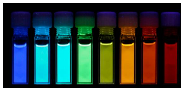
Figure 1. Photographic images of Indazo-Fluors 6a–6h in \text{CH}_2\text{Cl}_2 (excited at 365 nm under a UV lamp). Reproduced from ref 5b . Copyright 2016 American Chemical Society.
