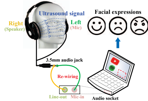
Figure 1: FaceListener recognizes facial expressions from the acoustic signal transmitted above the face skin surface.
