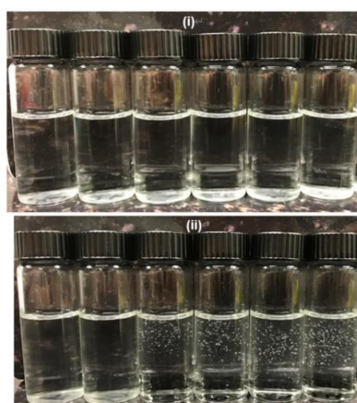
Figure 5. Photographs of remediation experiments (i) 5 mL of 0.02 wt% of 6CC mixed with 5 mL of varying concentration of Pb^{2+} (left to right: 5, 10, 25, 50, 100 and 250 ppm), (ii) 5 mL of 0.02 wt% of TCC mixed with 5 mL of varying concentration of Pb^{2+} (left to right: 5, 10, 25, 50, 100 and 250 ppm).
