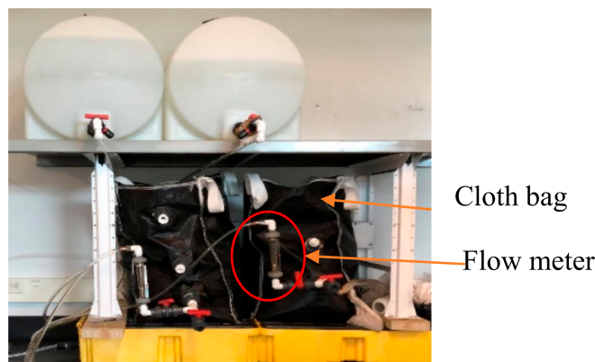
Figure 1. Biosand bag filtration setup.
