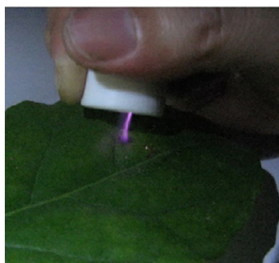
FIG. 26. Atmospheric plasma jet in direct contact with a plant leaf infected with pathogens. 151
