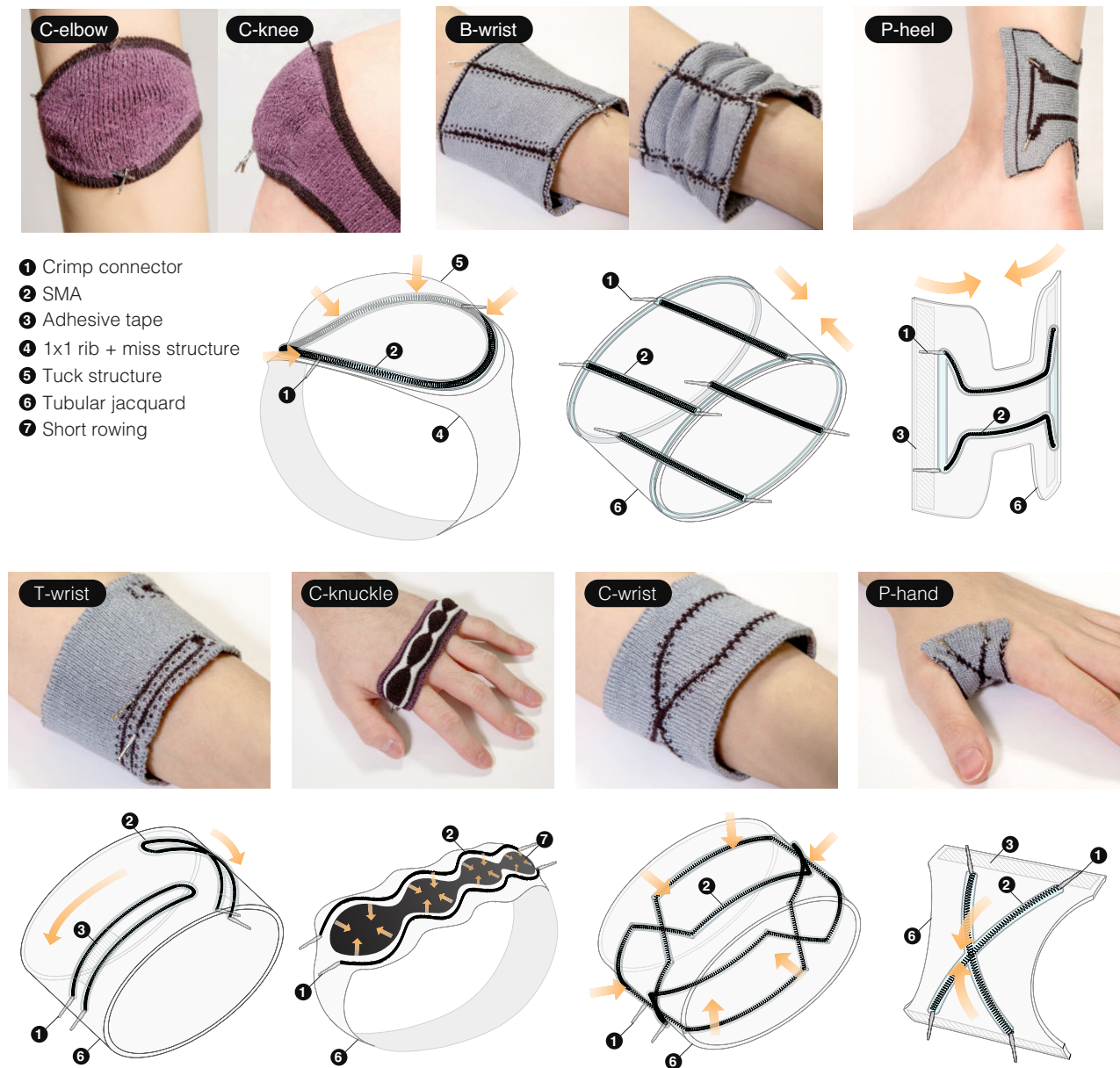
Figure 5: Summary of eight KnitDermis case studies. Depending on haptic feedback of interest, each case study variously configures design factors to conform to specific body locations. B-wrist and C-wrist adopt self-shifting mechanism whereas the remainder utilizes skin-shifting mechanism.
