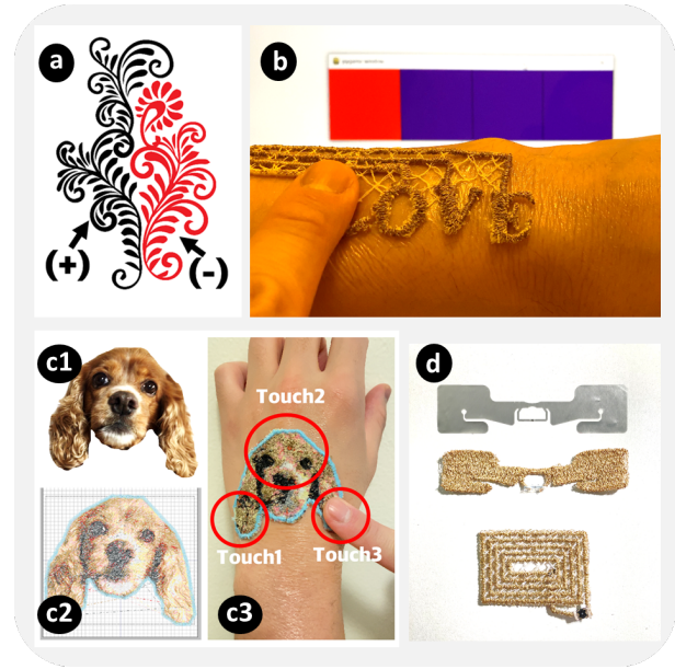
Figure 3: SkinLace applications (a) PCB design for SkinLace (b) four letters as capacitive touch electrodes, (c1-3) image for customized SkinLace, conversion into stitches, and fabricated result with three touch points, and (d) UHF RFID tag and NFC tag.
