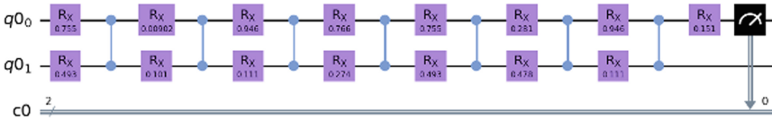
Fig. 10. Initial values for gradient parameter-shift circuit application
