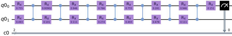
Fig. 8. The Cappelletti circuit in QisKit
