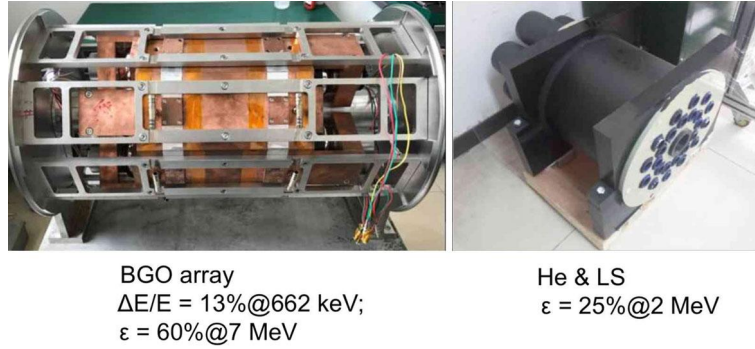
Fig. 2 The BGO and neutron detector arrays for JUNA
