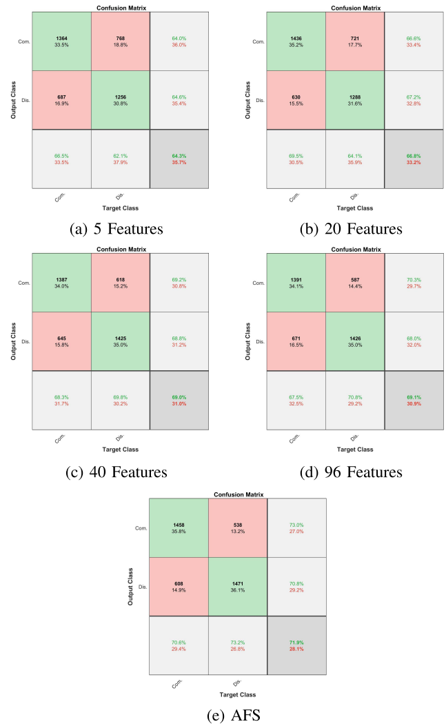
Fig. 8. Confusion matrices based on the testing results across all participants when using classifiers trained with different no. of features.
