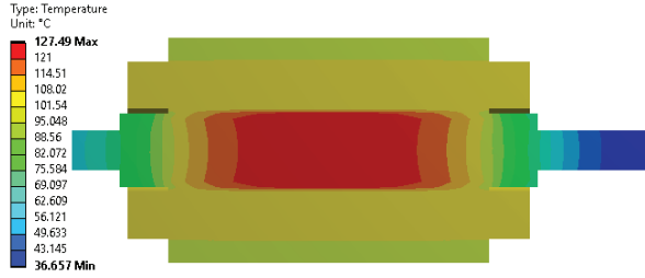
Fig. 8: Temperature distribution at rated condition.
