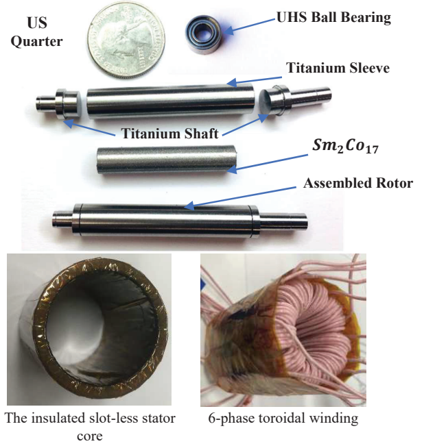
Fig. 13: UHS AMEBA rotor parts and assembly.
